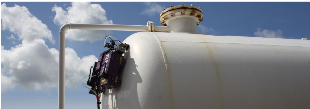
Figure 1 Automated Phased Array with Silverwing RMS2 and M2M Gekko
