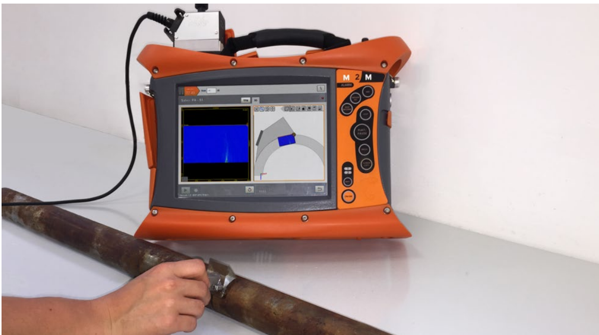
Figure 12 Small Bore PAUT Weld Inspection
