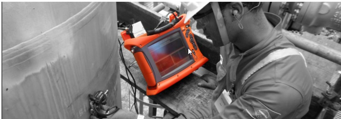
Figure 8 Phased Array with Gekko System
